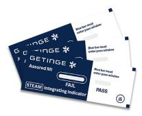
During steam sterilization, the chemical pellet of this Type 5 (Integrating Indicator) melts and migrates as a blue color along the paper wick. The migration is visible through a pass/fail window.
