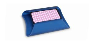
This Type 2 (Bowie-Dick test indicator) is designed for daily monitoring of pre-vacuum steam sterilizers operating at 132°C for 3.5 minutes to detect the presence of residual air.
